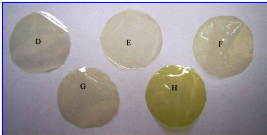
Figure 2. Typical pictures taken on films of ca. 25 \mu\text{m} stored for 60 days under different conditions: (D) control (a just formed film); (E) 4 °C, 0% RH; (F) 37 °C, 0% RH; (G) 23 °C, 0% RH; (H) 23 °C, 75% RH.
